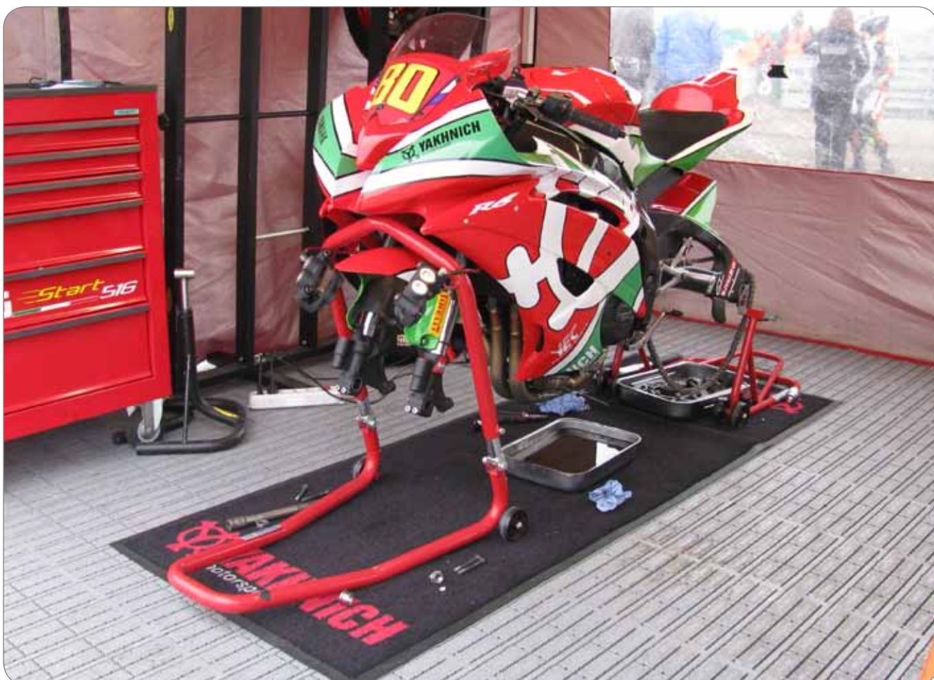
Above: A suitable environmental mat with absorbent top layer and liquid proof bottom layer. Circuit owners and organisers are encouraged to keep in stock a certain number of mats to sell or rent to those who, for any reason, do not have mats at events.
