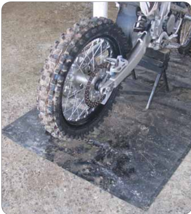
Above: Ordinary plastic sheeting does not provide proper protection, since it has no absorption qualities. Absence of an environmental mat creates a potential pollution risk.
