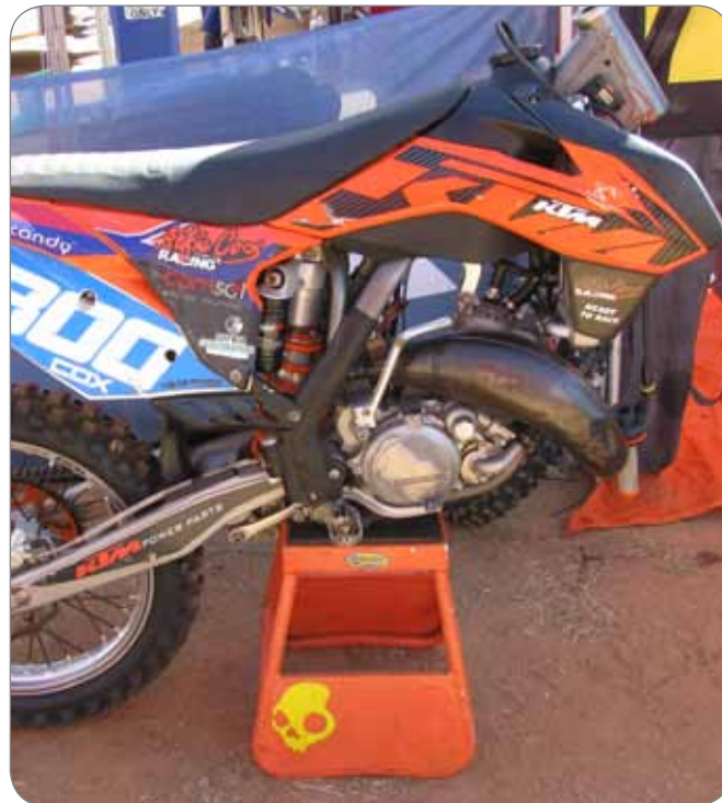
Above: Ordinary plastic sheeting does not provide proper protection, since it has no absorption qualities. Absence of an environmental mat creates a potential pollution risk.
