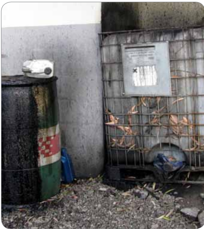
Above: Inappropriate storage of used oil in leaking and rusted containers
