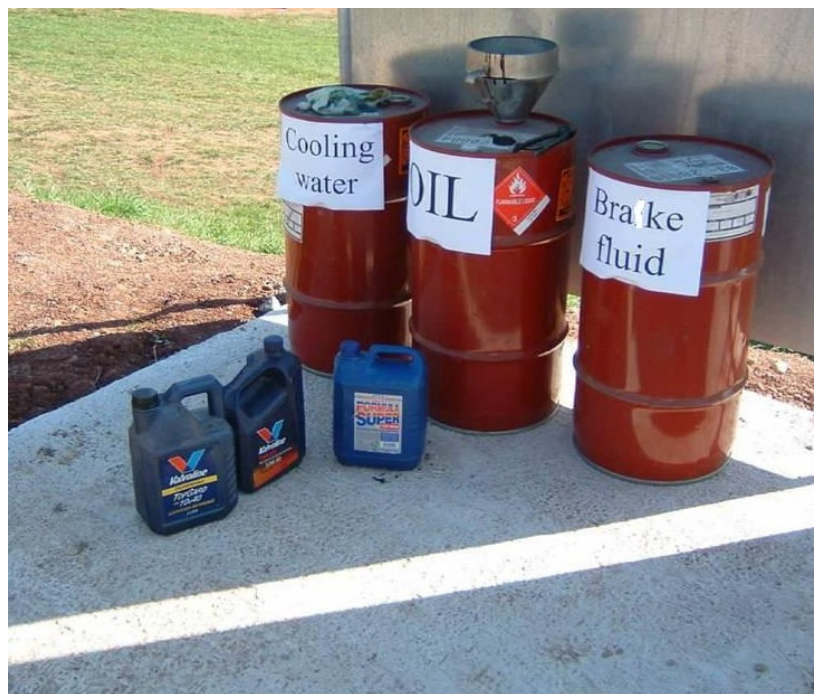
Above: Sturdy and functional containers for disposal of used vehicle fluids and filters. Note positioning on non-porous surfaces and provision of funnel.
